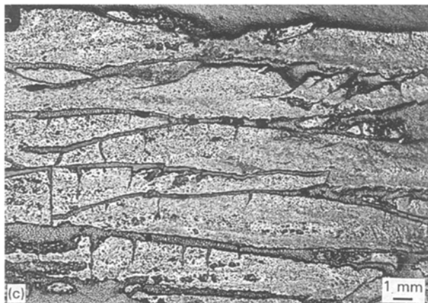
Figure 11 TiC-Al 2 O 3 microstructures using Al 2 O 3 as a diluent to control the reaction rate (a) 5 wt %, (b) 10 wt % and (c) 15 wt %.
